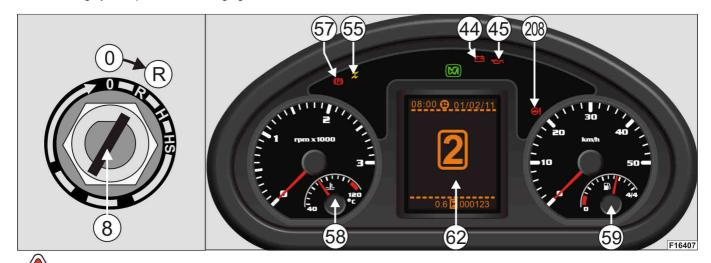
CAUTION! Should the indicators fail to function as indicated, immediately switch off the engine. If the crab steering warning light (55) is lit, use the appropriate lever to reset normal conditions.
