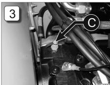
CAUTION! Oil change in the hydrostatic transmission shall be performed by skilled and qualified personnel. Only use hydrostatic oil listed in the section"FUEL AND LUBRICANTS". Check oil level in the tank quite frequently and, if necessary, top it up.
