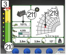
To restore safe operating conditions (both indicator (219) and LED graphic bar (210), first retract the telescopic boom.
